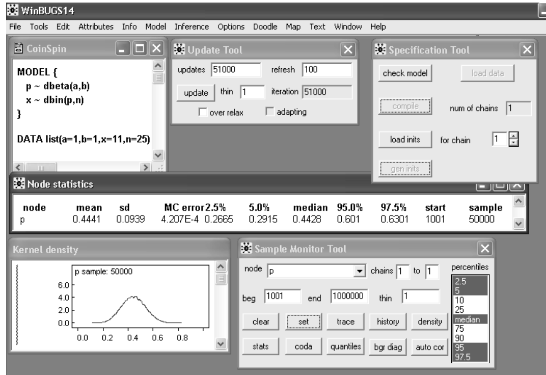
Figure B.10 A complete WinBUGS session. The posterior distribution of p , the rate of occurrence of heads in coin spinning, is approximately normal with \mu = 0.444 and \sigma = 0.094 .
