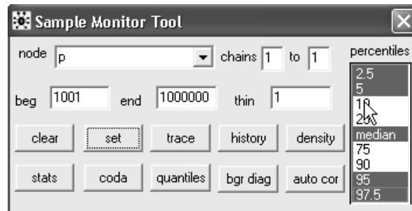
Figure B.9 The Sample Monitor Tool. The user has requested five percentiles. The arrow cursor is positioned to select the 10th percentile (ctrl-click the left mouse button).
